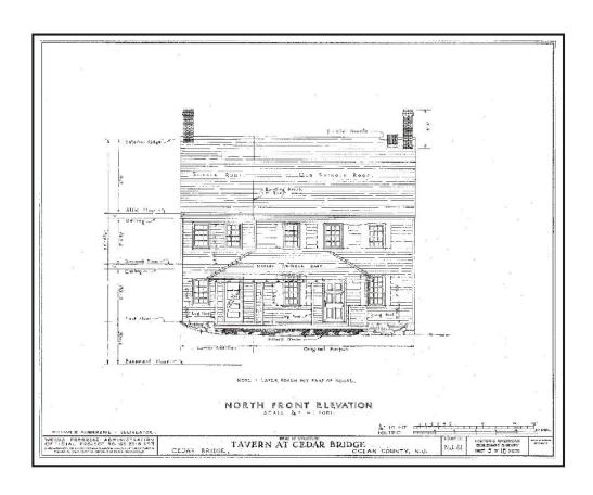
**Figure 3.6:** 1938 HABS, North Front Elevation of the Tavern at Cedar Bridge (Survey No. N.J. 41). Note original section of the structure (Right two-thirds).
