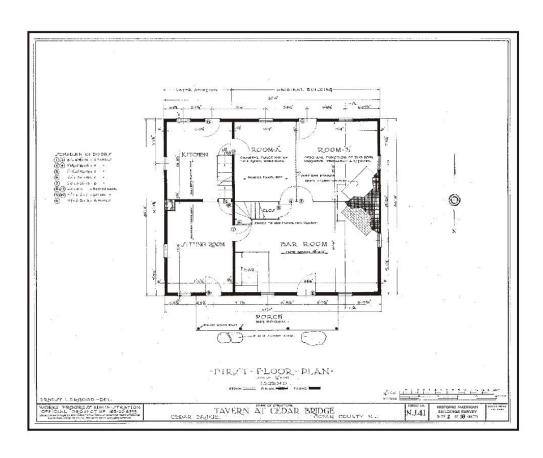
**Figure 3.9:** 1938 HABS. First Floor Plan of the Tavern at Cedar Bridge (Survey No. N.J. 41).
